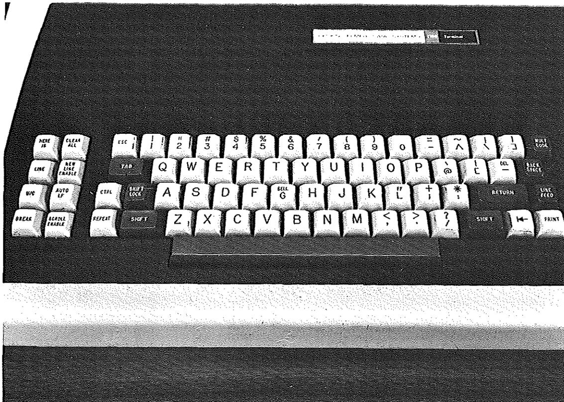
Photograph 2-14: Perkin-Elmer Keyboard and Configuration Buttons
